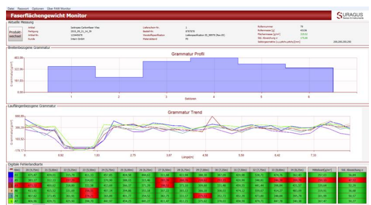
Fiber areal weight monitoring of 7 lanes. Roll report listing locations with ok and not-ok material.
