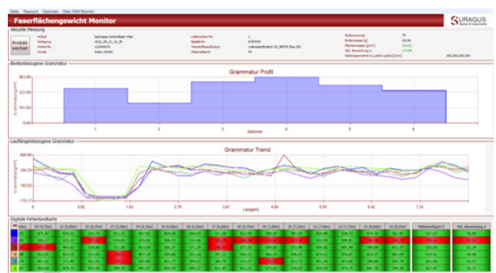
Fiber Areal Weight monitoring of 6 lanes. Roll report listing locations with ok and not-ok material.
